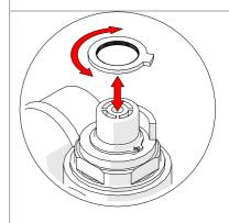
Remove the lower brass ring (temperature setting ring) and rotate the brass ring clockwise to increase temperature or anticlockwise to decrease.
